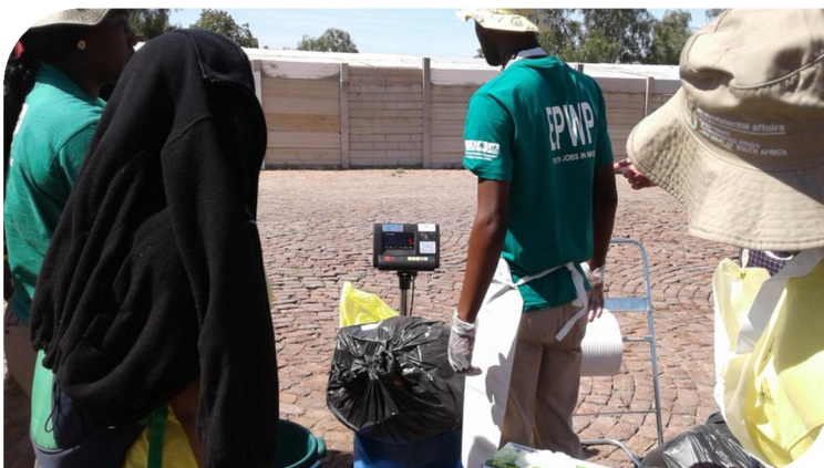
Figure 2.6: Unopened black bag being weighed and mass on label being recorded
